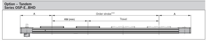
\*\* Order stroke = required travel + KM min + 2 x safety distance
