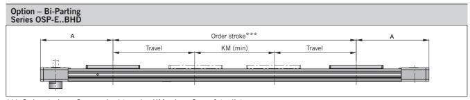
\*\*\* Order stroke =  $2 \times \text{required travel} + \text{KM min} + 2 \times \text{safety distance}$
